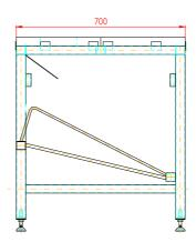
Working table for meat – boning is made from stainless steel material and equipped with plate from health-unexceptionable material – *nierolen*. There are two holes cut out plate, which are used for meat dropping in boxes, which are placed in holders in lower part of the table. Adjustable feet allow stable table settlement. This working table is most often used as a part of boning conveyer and is fixed to its sides.
